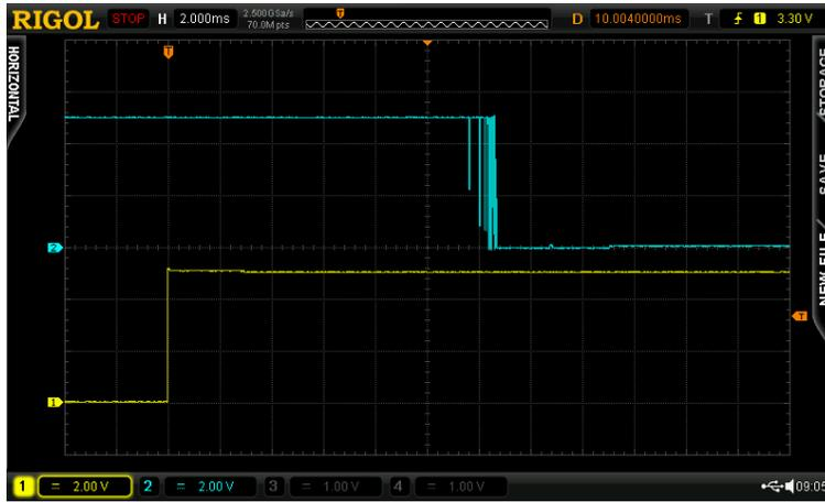
Figure 10: Relay contact switching,  $V_B$  - yellow line,  $V_Z$  - blue line
